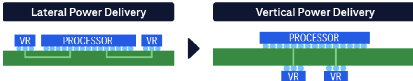
Figure 12. Lateral Power Delivery vs Vertical Power Delivery
